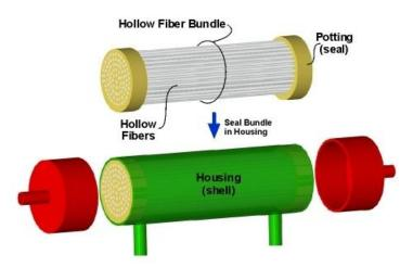
Therefore the rate of gas transfer across the membrane is proportional to the gas permeability coefficient, the membrane surface area, the trans-membrane gas partial pressure difference, and inversely proportional to the membrane thickness. Thus gas transfer across a membrane increases with increased gas permeability coefficient, increased surface area, increased transmembrane gas partial pressure and decreased membrane thickness.
