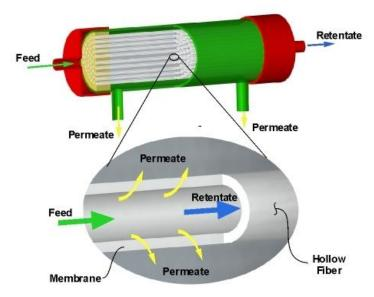
Gas Separation. Although the permeability ratio for two gases in a binary gas mixture provides a gross estimate for the ratio of permeate flow for the two gases, actual measurements show that the interaction of a gas mixture on the membrane can affect permeation rates. Moreover feed and permeate pressures can also affect permeation rates as the membrane structure can change under pressure. The **separation factor** is a
